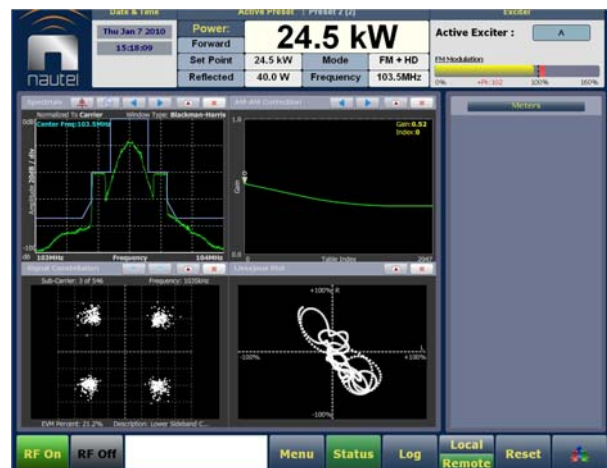
AUI showing built in Spectrum Analyzer
